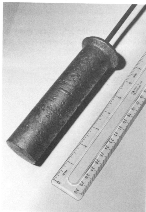
Figure 2: Picture of ferromanganese cylinder 3.8 cm in diameter and 15.2 cm in length.
