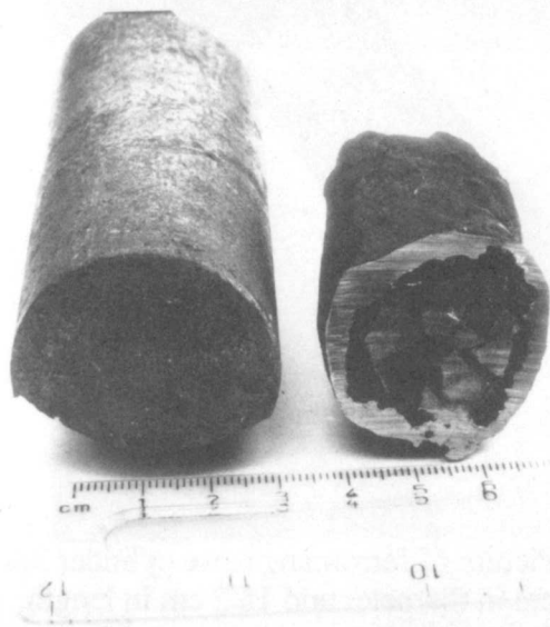
Figure 4: The cylinder on the left is shown before immersion in liquid steel, and on the right is a cross section of a similar ferromanganese cylinder following immersion for 20 seconds in a steel bath having an initial superheat of 130^{\circ}\text{C} . Initial cylinder diameter was 3.81 cm.
