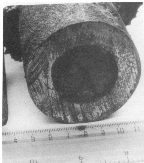
Figure 3: Cross section of a ferromanganese cylinder following immersion for 30 seconds in a steel bath having initial superheat of 30^{\circ}\text{C} . Initial cylinder diameter was 3.81 cm.
