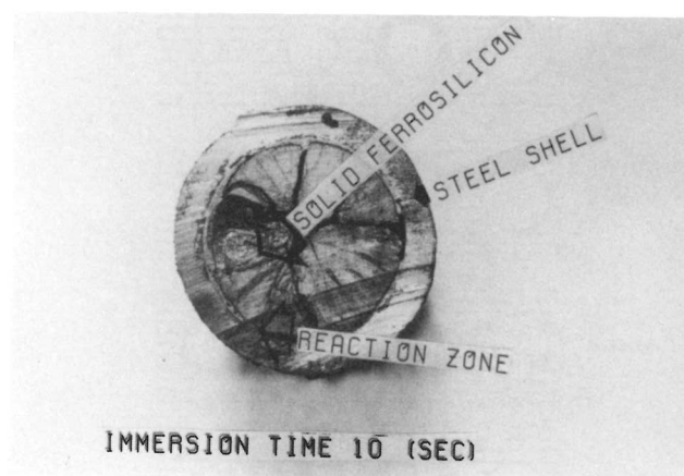
Figure 6: Sectioned 50 wt% ferrosilicon cylinder showing encasing steel shell and extent of reaction zone following immersion for 10 seconds.
