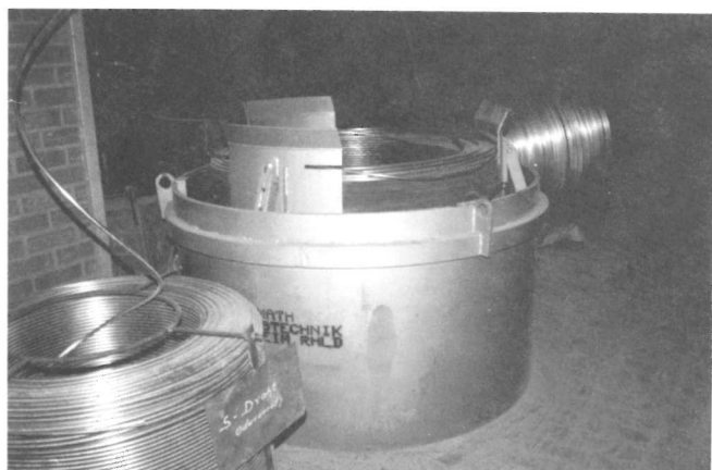
Fig. 29 Static pay off device for vertical uncoiling
