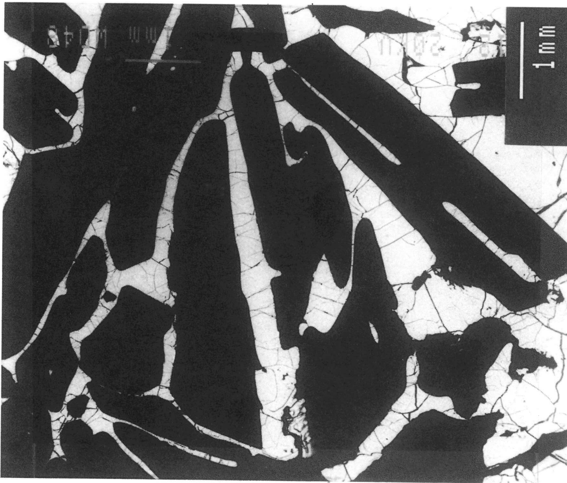
Picture 4 shows the lowest solidification rate with 0.21°C/min and a grain diameter of 784 \mu\text{m}
