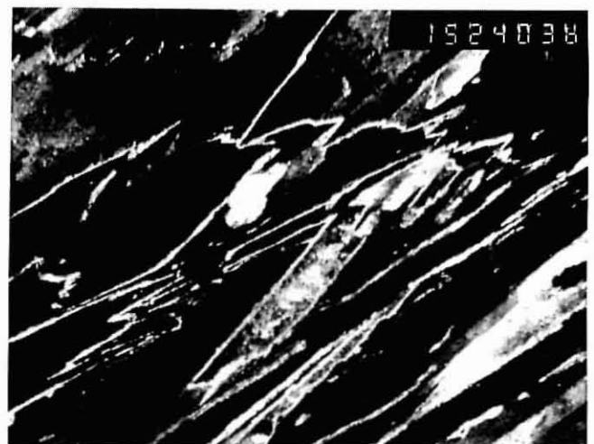
FIGURE 8. Transmission electron microscope (TEM) showing the films of retained austenite (white) surrounding martensite laths (dark)
