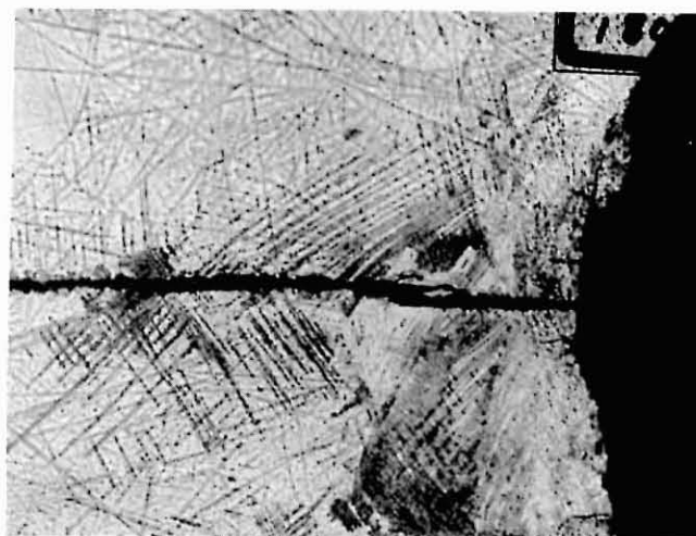
FIGURE 12. At low applied \Delta K levels ( \Delta K < 10 \text{ MPa}\sqrt{m} ), initiation occurred at single sites only. (AEC-316LNG 150 x magnification)
