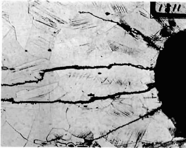
FIGURE 13. At higher delta-K levels ( \Delta K > 12 \text{ MPa}\sqrt{\text{m}} ), multi-initiation is evident. (AEC-316LNG, 150 x magnification)
