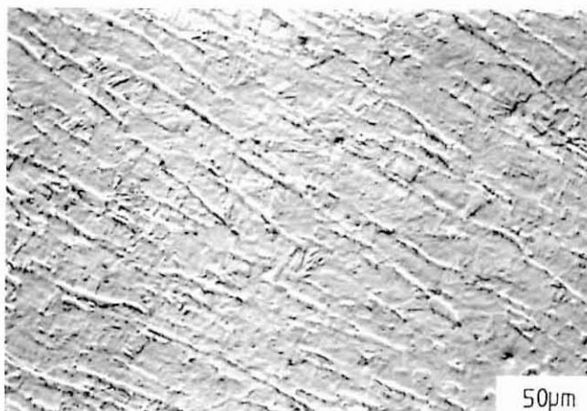
FIGURE 11. Alloy E5 exhibits residual \delta -ferrite stringers in a martensitic matrix (solution-treated)
