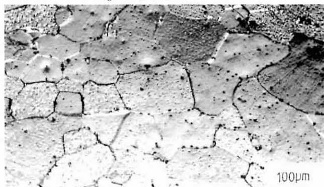
FIGURE 2. Large-grained ferrite microstructure of alloy E1 (1000 °C)
