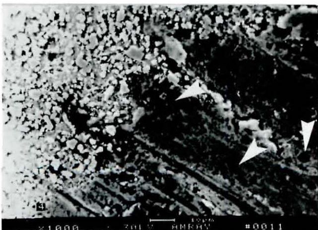
FIGURE 11. Tapered section of specimen No. 4 (SEM) – pits formed by spalled particles of carbide
