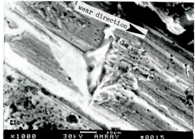
FIGURE 12. Worn surface of specimen No. 4 (SEM) – fractured and embedded abrasive particle stopped by carbide
