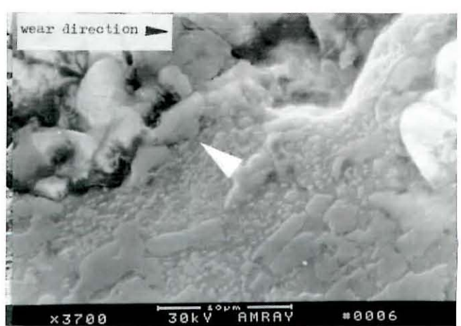
FIGURE 13. Normal section of specimen No. 4 (SEM) – moving abrasive particle stopped by carbide
