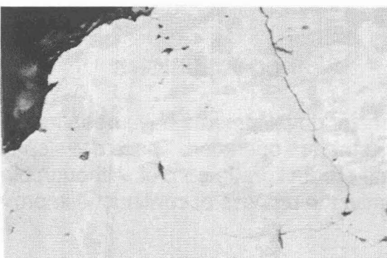
Plate 5: Section showing different intermetallic phases existing in sample T5M1
