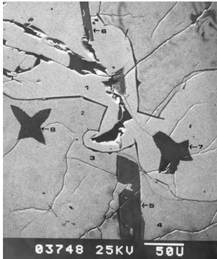
Figure 1. Photomicrograph of charge chrome alloy showing some typical Ti-containing inclusions [7] [1,2 = (Cr,Fe) carbide; 3 = \sigma phase (Cr,Fe) alloy containing 15% Si and 0.2% Ti; 4 = (Cr,Fe) silicide; 5,6 = Ti sulphide (65% Ti); 7 = Ti carbonitride (55% Ti)].
