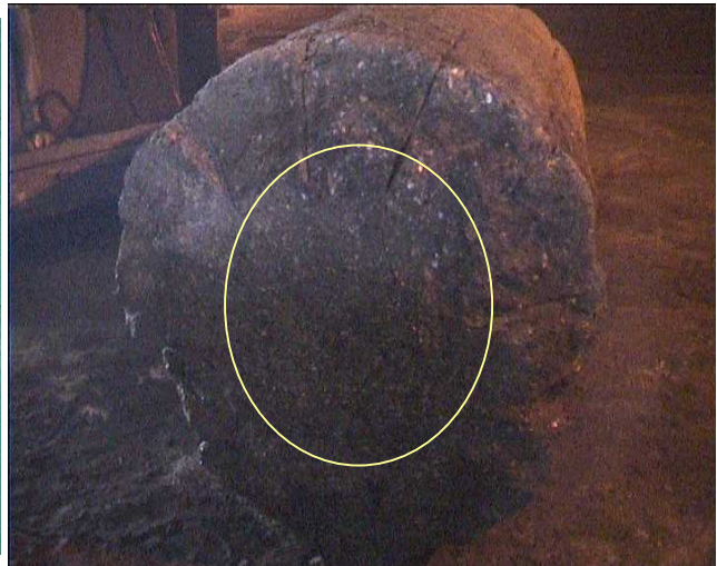
Figure 5. Electrode B stub ( \pm 2.2 m long) with evidence of segregation of larger aggregate from finer aggregate/pitch binder at the electrode periphery.
