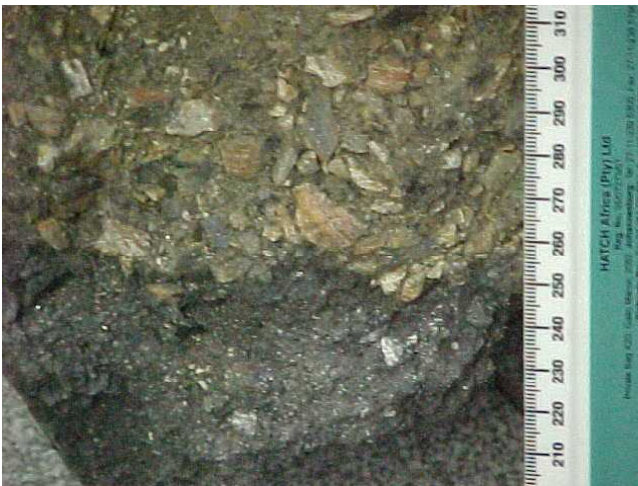
Figure 4. Close-up of Electrode A shows significant paste segregation into brittle carbonised pitch binder and a coarse calcined anthracite aggregate.
