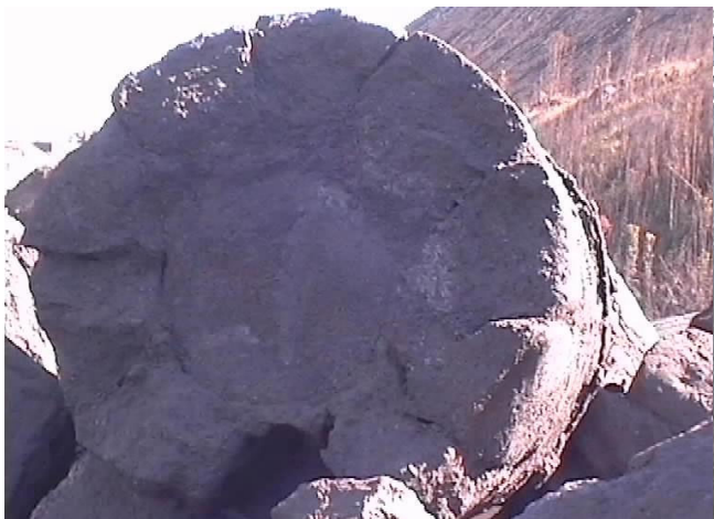
Figure 8. Remarkable broken Electrode D stub, showing the outline of a paste cylinder at the electrode core. Sure signs of inadequate control of paste addition, paste levels and baking.
