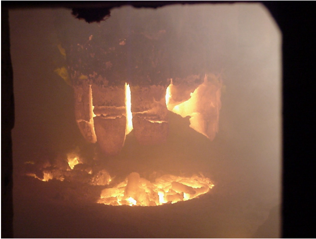
Figure 10. 140 cm diameter Electrode F showing poor baking, fluted attack between fins and circumferential cracks and break.
