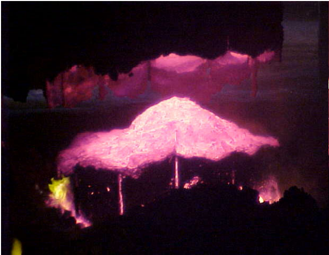
Figure 2. The shape of the break cusp may suggest an “over-baked” electrode, but slipping in excess of 36 cm per day contradicts this as a cause of the break (Electrode A). Conditions of low soft paste level and paste volatilisation were noted.
