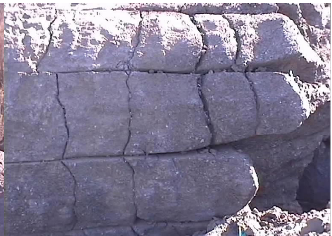
Figure 9. Regularity of circumferential cracks around Electrode E may relate to a daily paste loading event. Associated with practices of dropping of paste cylinders and overloading hard paste.
