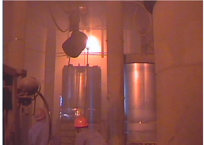
Figure 11. Paste slinging and loading practice sub-standard with every cylinder dropped into the electrode column.
