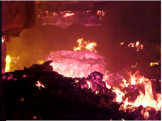
Figure 3. The shape of the break cusp may suggest an “over-baked” electrode, but slipping in excess of 40 cm per day again contradicts “over-baking” as a cause of the break (Electrode B).
