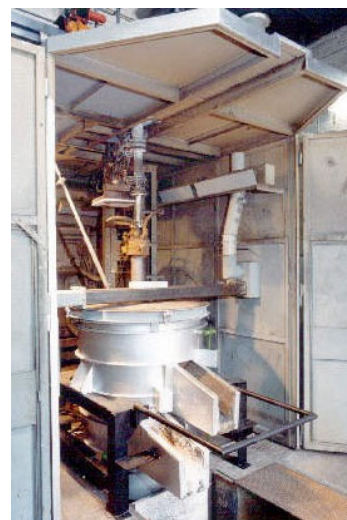
Figure 12. 520 kVA test furnace in Aachen/Germany.
