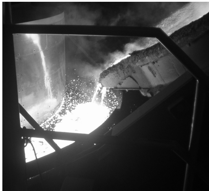
Figure 7. Operation of casting onto the copper carousel.
