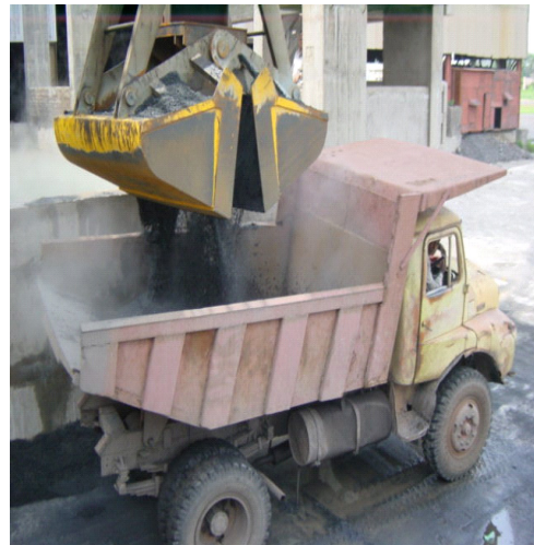
Figure 11: Granulated slag disposal
