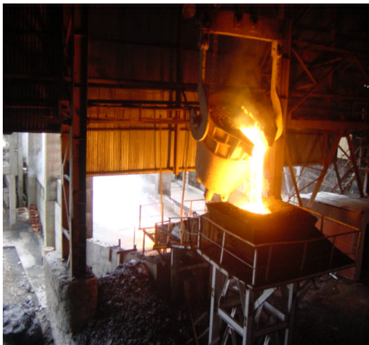
Figure 10: Granulating of liquid slag
