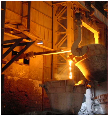
Figure 4: Skimming of floating slag
