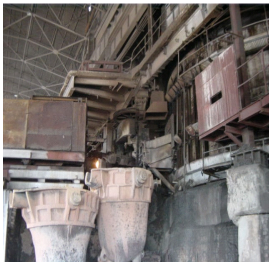
Figure 2: Movable tapping platform close to taphole
