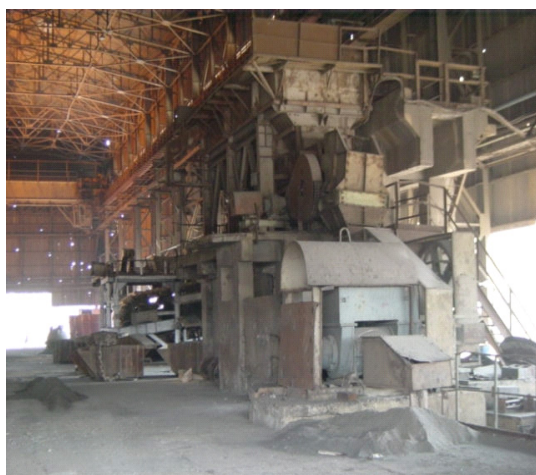
Figure 8: Jaw crusher for metal crushing
