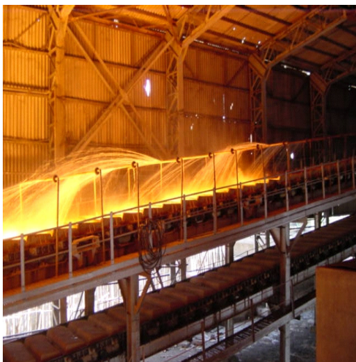
Figure 6: Metal solidification with water showers
