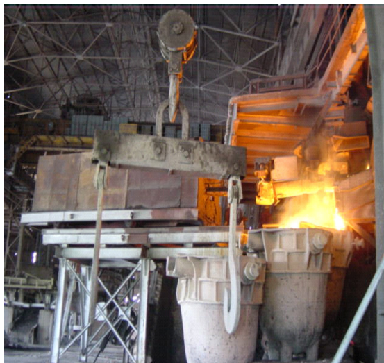
Figure 3: Movable tapping platform away from taphole
