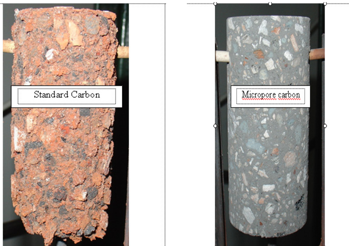
Figure 2B: Oxidation of standard carbon (A) versus micropore carbon (B) - samples after testing at Figure
