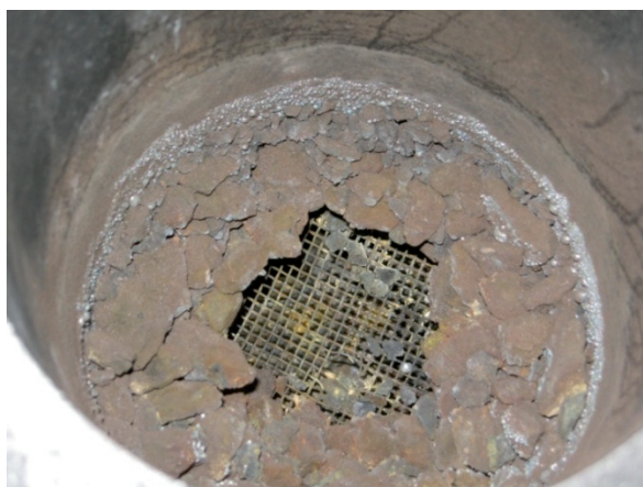
Figure 5: The layer of charge materials filled with metallic Zn and ZnO. The experiment was performed at 1100 °C and 1 h of keeping time.
