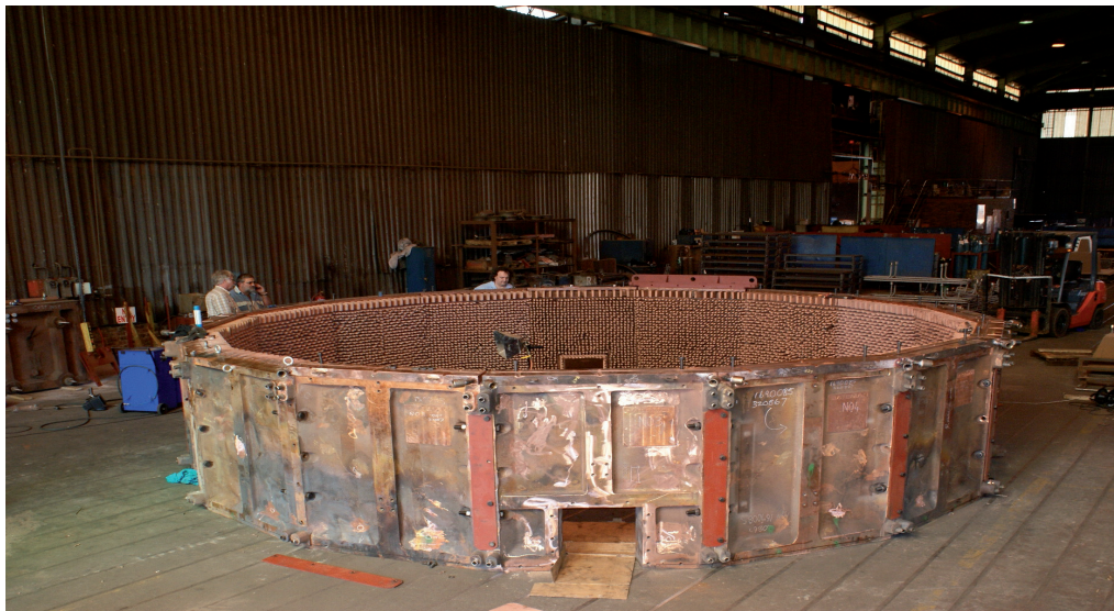
Figure 10: Shop assembly of the 12 MW DC Furnace CFM side wall cooling panels.
