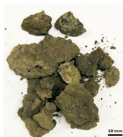
Figure 2: The typical example of charge agglomeration due to alkali deposition
