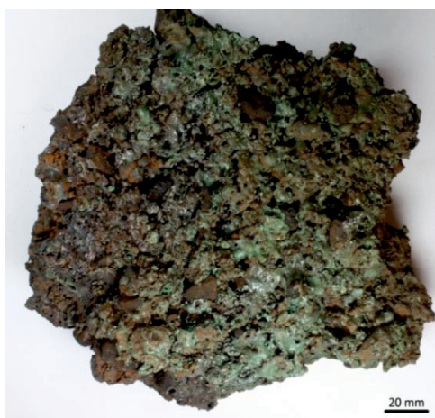
Figure 1: The typical example of charge agglomeration due to slag eruption
