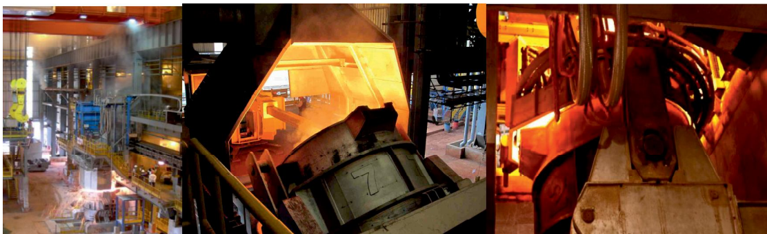
Figure 3: Refinery equipment (left: oxygen blowing station; centre: deslagging stand; right: ladle furnace)
