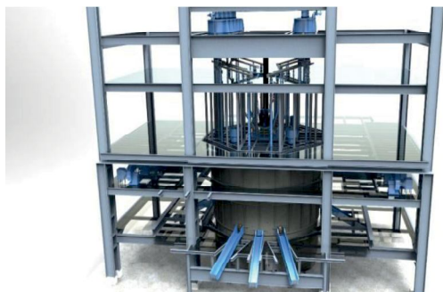
Figure 6: Illustration of the DC-furnace as being built for Kazchrome/Kazakhstan [5]
