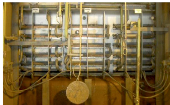
Figure 7: Side wall copper cooling system [7]
