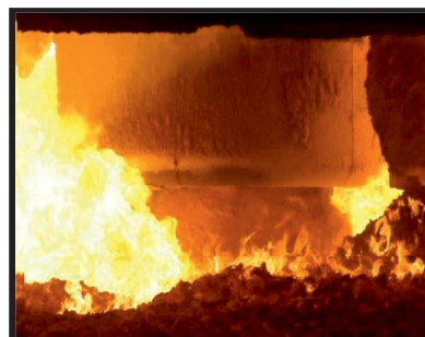
Figure 5: Lower part of the electrode column
