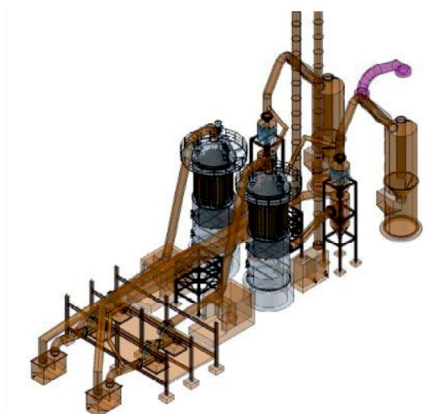
Figure 16: Wet scrubber gas cleaning plant for closed type submerged arc furnaces
