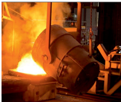
Figure 1: Pouring of silicon from the ladle to the mould. The casting process may create smoke and dust from silicon surfaces at temperature above or near the melting point
