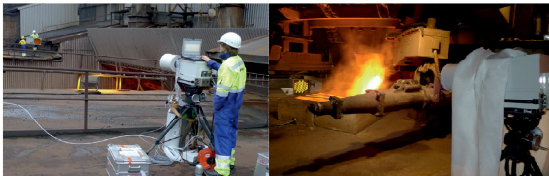
Figure 1: OP-FTIR application over slag pit (left) and during tapping (right)
