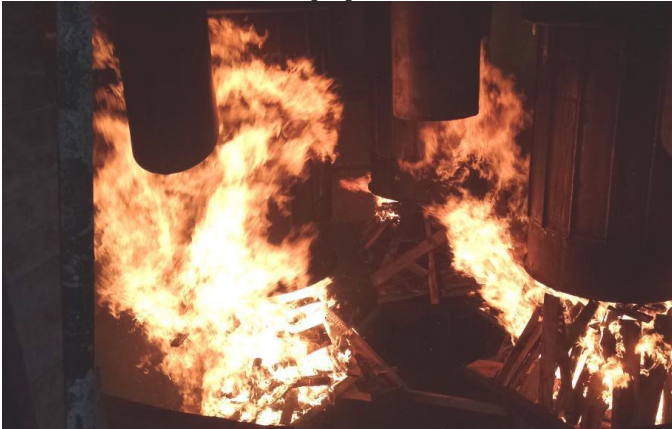
Firing wood to heat and soften electrode paste
