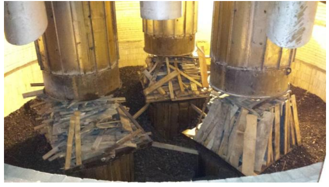
Wooden charge between electrode
