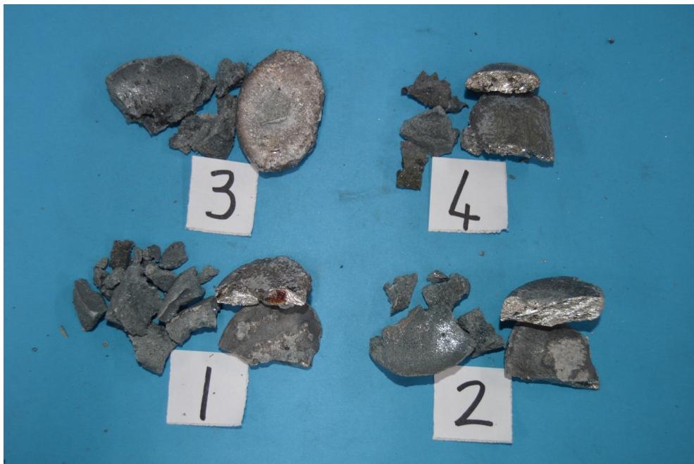
Figure 9: An example of the bulk alloy pellet that forms and is collected from a smelting test (bright grey/silver = alloy)
