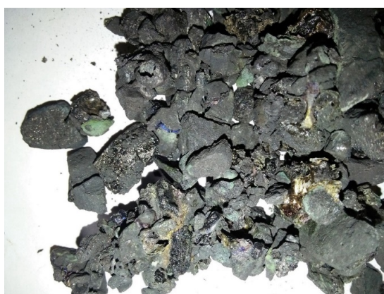
Figure 5: Pre-reduced Venarch sample at 1100°C in 50%CH 4 -50%Ar for an hour
