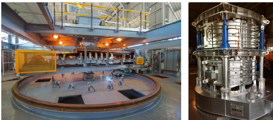
Figure 6: Day bin rotating conveyor with cartridge filters and preassembled Metix slipping device
