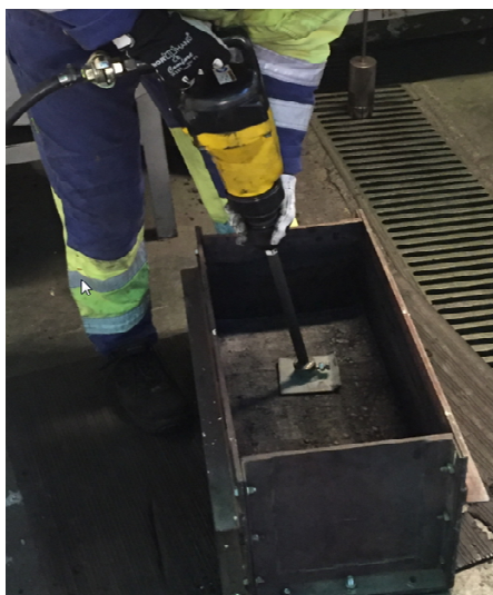
Figure 3: A steel mould, and equipment for ramming of carbon and SiC materials
