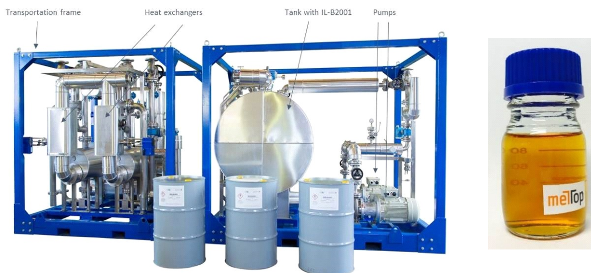
Figure 3: Basic design of an ILTEC system, as installed at ArcelorMittal Bremen GmbH in Germany (left); and photograph showing the optical appearance of the ionic liquid IL-B2001
