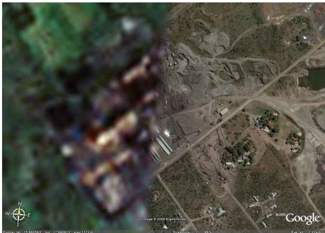
Figure 9: Image of Hernic Ferrochrome plant in Brits, South Africa, showing contrast between high and low resolution coverage [Image ©2006 DigitalGlobe]
